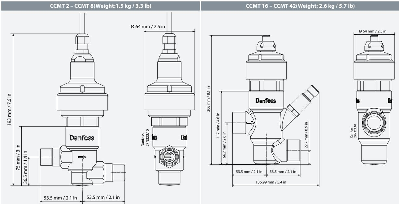
CCMT 16 – CCMT 42 (without integrated pressure transmitter)
