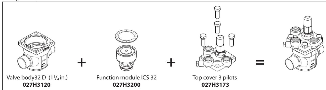
Figure 36: ICV 32 valve body w/different connections
