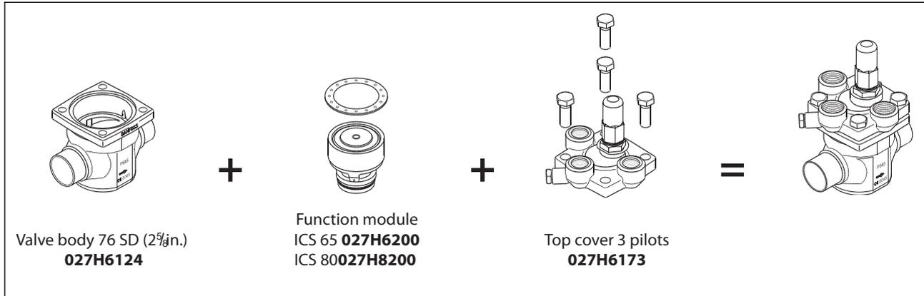
Figure 57: ICV 65 valve body w/different connections
